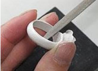
13) Trim any burrs on the inside of the ring and sand the sides with a medium fine file. Smooth the entire piece with a red sponge sanding pad (#320-600), and fire.
