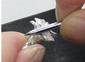
14) Polish the entire piece with a stainless steel brush and make a shiny finish on the edges of the ring and rose petals. Finally, polish using a polishing cloth and some silver polish and finish.
