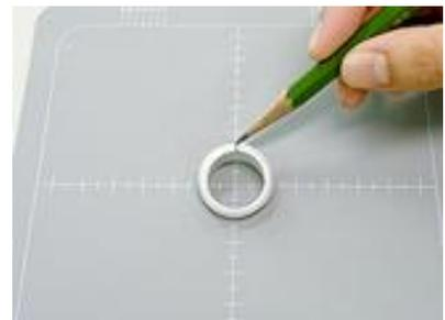
3) Place the piece on the center of the work surface, and draw a center line with a pencil on the ring top.
