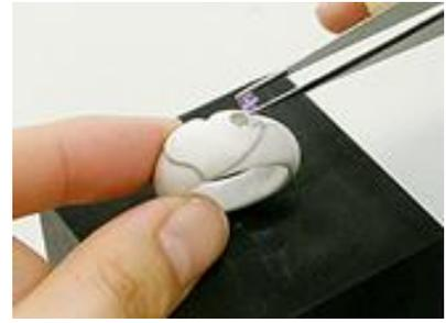
9) Put a small amount of Paste Type to attach the synthetic stone, dry and fire.
