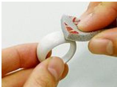
2) Smooth the sides with a medium fine file and #320 grit sandpaper, and the surface and inside of the ring with the file and a red sponge sanding pad (#320-600).
