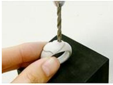
8) Open a shallow hole on the upper right heart with a  $\phi$  3 drill bit.
