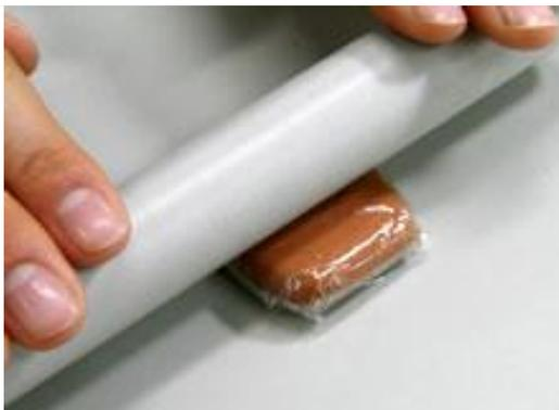
**Tip:** Oxidized film will be made on copper clay due to exposure to the air. The best storage method to prevent oxidized film is by wrapping the copper clay and plastic wrap tightly without any air pockets and then roll out the clay with a roller to bind them more closely together.
