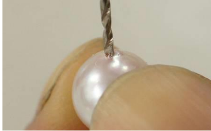
11. Expand the hole sizes of three pearls with a \phi 1.0mm drill bit.
