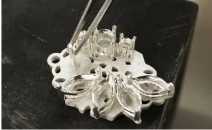
10. Attach the 3 wires on the space of the back. After drying completely, put the piece in a kiln and ramp up from room temperature to 800C/1472F.
