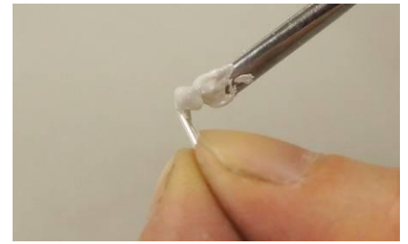
9. Put plenty of Overlay Silver Paste on the tip of silver wire.
