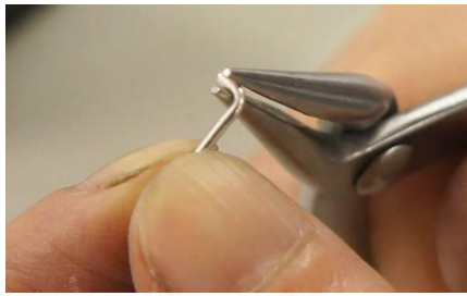
8. Cut the \phi 0.1mm silver wire into 3 wires x 10mm. Bend the tip into an L-shape like in the image above.
