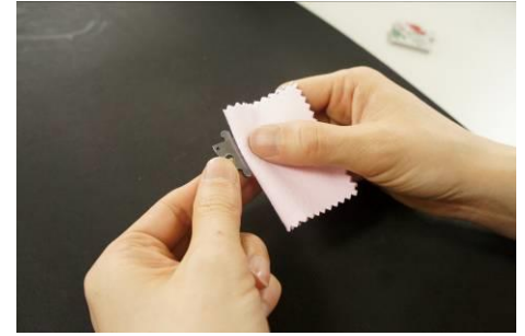
22) Rinse well with water, wipe off with some tissue and polish the surface lightly with a polishing cloth so as not to remove all of antique effect.
