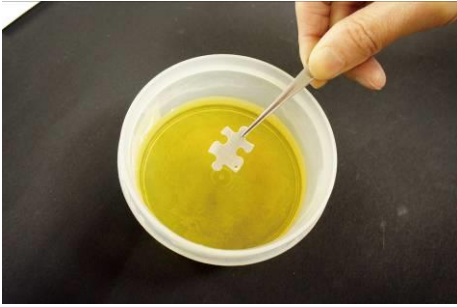
20) For the antique finish, pour some hot water (70-80C/), add 3-4 drops of liver of sulphur solution and stir well. Then, put the piece in.
